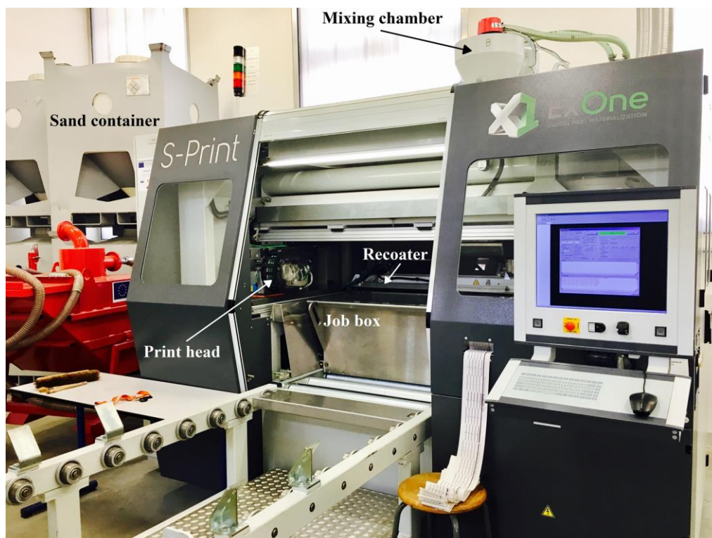
Fig.3 3D sand printer used in the present experiments
