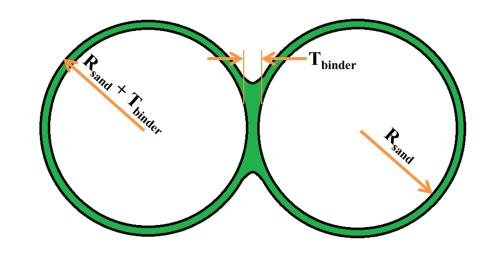
Figure 7. Resin bonding bridge of adjacent sand particles
