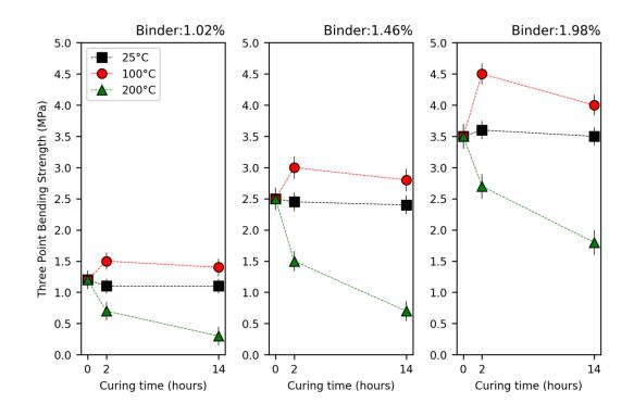
Figure 6. Effect of curing parameters on 3PB strength
