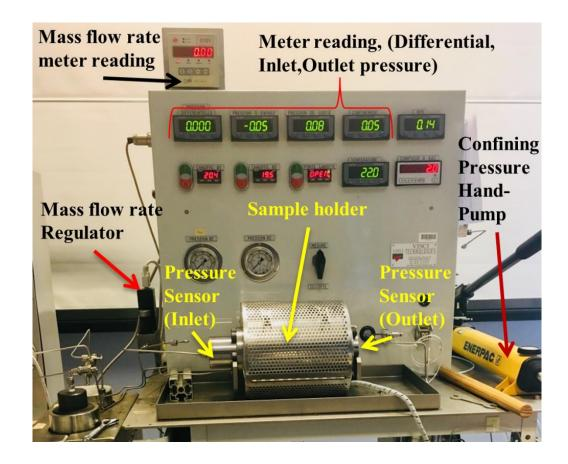
Figure 4. Perm-meter setup
