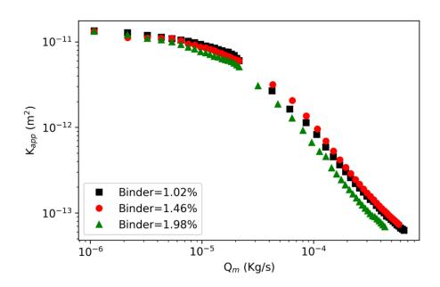
Figure 10. Relationship between apparent permeability and mass flow rate for uncured
