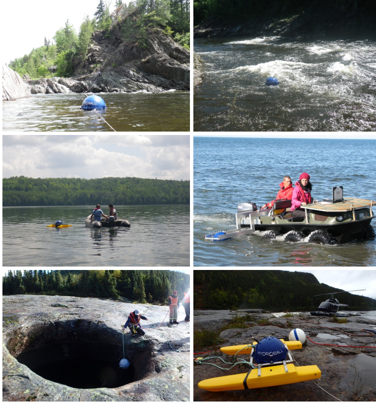
Fig. 2 Some applications of the HydroBall system: Top left: Transect of a river (Rimouski river) ; Top right: Riverbed survey (Rimouski river) ; Middle left: Deployment from an inflatable (Anguille Lake) ; Middle right: Deployment from an amphibious vehicle for beach profiling (Anse au Lard) ; Bottom left: Survey in a confined area (Romaine river) ; Bottom right: Deployment from an Helicopter for dangerous areas surveys (Romaine river).
