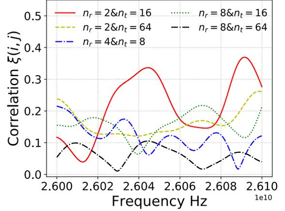
Fig. 3: Correlation over 100 MHz bandwidth at 26GHz
