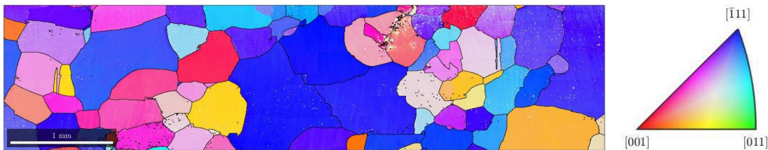
Figure 1: Grains orientations as obtained from EBSD measurements. Grains are colour-coded according to the adjacent key Inverse Pole Figure.
