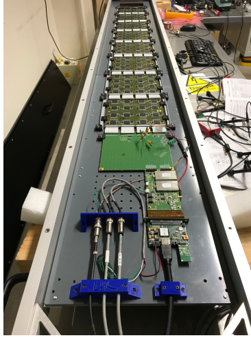
Figure 1: Assembled long slab with 8 ASUs.
