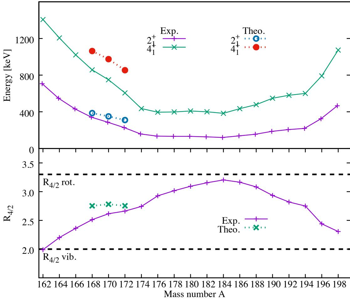
FIG. 1. (Color online) The excitation energy systematic of the  $2^+$  and  $4^+$  yrast states in the osmium isotopes in the upper panel. The structural benchmark  $R_{4/2} = E_{4_1^+}/E_{2_1^+}$  is presented in the lower panel together with the empirical limits for rotation and vibrationnal nuclei. The theoretical values for  $^{168,170,172}\text{Os}$  are a part of this work.
