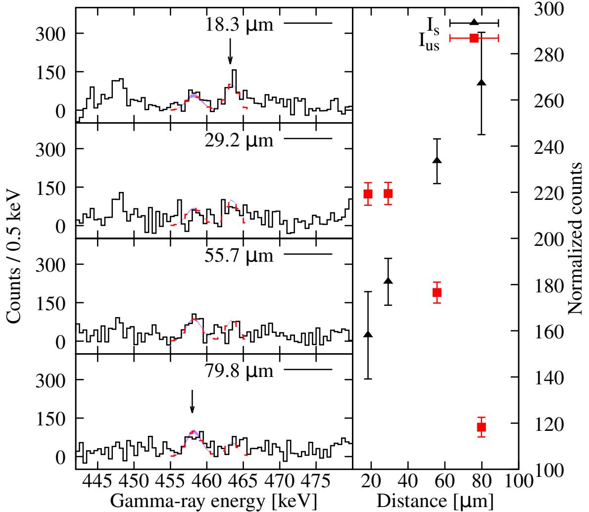
FIG. 5. (Color online) Same as Fig. 4 for the  $4_1^+ \rightarrow 2_1^+$  transition at 133.5 degrees obtained by gating on the  $6_1^+ \rightarrow 4_1^+$  in-flight transition.
