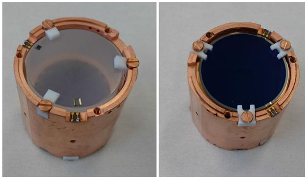
**Fig. 4** An assembled CUPID-Mo module. On the left: view from the top, the semi-transparent crystal surface where the NTD and heater are located. On the right: view from the bottom, germanium LD with SiO coating (dark blue internal circle); the 2 mm on the edge of the wafer (17% of the area) are uncoated
