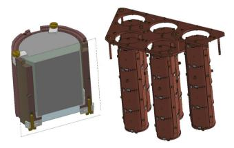
Fig. 1 Rendering of a CUPID-Mo single detector module (left) designed to hold a  $\text{Li}_2^{100}\text{MoO}_4$  scintillating element. A module is comprised of a crystal of size  $\oslash 44 \times 45$  mm and a Ge wafer of  $\oslash 44 \times 0.175$  mm. The full 20-detector bolometric array is arranged in five suspended towers containing four detector modules each (right)
