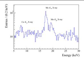
Fig. 9 Energy spectrum of CUPID-Mo light detector LD2 after a 33 h  $^{60}$ Co irradiation in the EDELWEISS-III set-up. The Mo K<sub> $\alpha$ </sub> X-rays are used for the LD calibration
