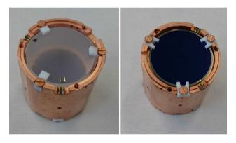
**Fig. 4** An assembled CUPID-Mo module. On the left: view from the top, the semi-transparent crystal surface where the NTD and heater are located. On the right: view from the bottom, germanium LD with SiO coating (dark blue internal circle); the 2 mm on the edge of the wafer (17% of the area) are uncoated
