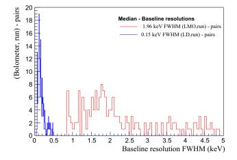
Fig. 11 Baseline resolution (FWHM) distributions for 183 (LD, run) and 189 (LMO, run) pairs. LMO 2 and LD 3 are rejected, as are periods with atypical noise
