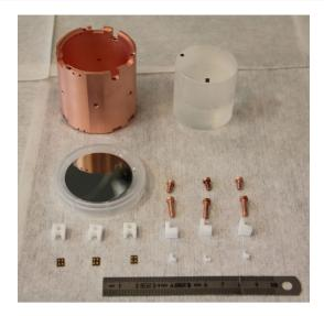
Fig. 3 All components used to assemble a CUPID-Mo single detector module: a copper holder, a  $\text{Li}_2^{100}\text{MoO}_4$  crystal with glued NTD and heater, a Ge LD with NTD, the copper screws, the PTFE spacers and fixing elements, the Kapton foil with golden pads. Note that the reflecting film is not shown here
