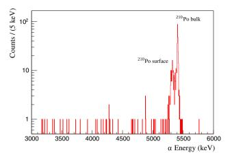
Fig. 17 Summed alpha region using 19/20 detectors. No RLY cut applied. (For details see text.)
