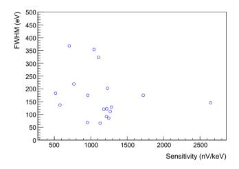
**Fig. 10** The baseline resolution versus sensitivity for 18/20 Ge LDs operated in the CUPID-Mo experiment at 20.7 mK. One detector is discarded due to having a different NTD (LD 3), while the second is not operational( LD 7, see text)
