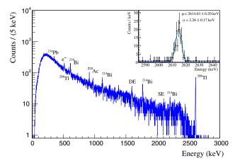
Fig. 13 Summed calibration spectrum for  $19/20 Li_2 MoO_4$  bolometers. All the major peaks have been labeled. The inset shows a fit of the  $^{208}$ Tl  $\gamma$  peak at 2614.5 keV
