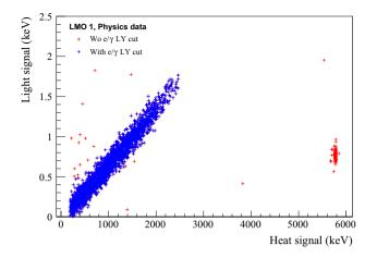
Fig. 15 Light yield versus heat signal scatter-plot using 11 days of physics data from LMO 1. The presented detector has the highest <sup>210</sup>Po contamination to illustrate best the distributions of  $\alpha$  and  $\gamma$  events and the scintillation light quenching for  $\alpha$  events
