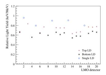
**Fig. 14** Relative Light Yields for all of the  $Li_2^{100}MoO_4$  crystals. The differences in RLY trace the expected light collection efficiencies due to the design of the towers, see Sects. 2.5 and 2.6
