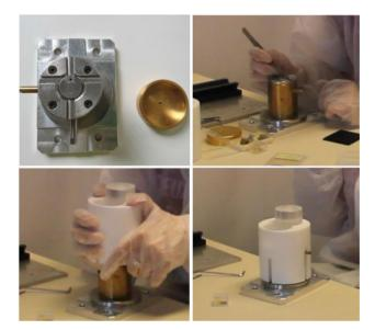
Fig. 2 The tool for gluing the sensor (top left) together with the cap to provide a 50  $\mu$ m gap. The process of gluing is shown in the three other photos: NTD placement (top right) and placement of the crystal (bottom panels)
