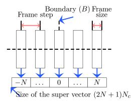
Figure 4: Construction of a super vector. We consider N non overlapping frames to the right and N non overlapping frames to the left of a boundary. In addition, we take into account the frame centred on the boundary. The (2N + 1) acoustic vectors of these (2N + 1) frames form the super vector.
