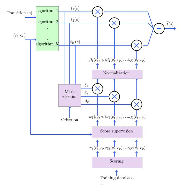
Figure 1: General scheme for computing  $\hat{t}(s)$  by linear fusion of segmentation marks. We have  $\delta_k$  equal to 1 if  $k \in A$ , where A is the index set of the selected marks, and 0 otherwise
