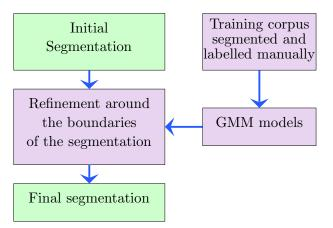
Figure 3: The different steps of refinement by boundary-model
