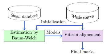
Figure 2: Segmentation by HMM based on a small corpus manually segmented
