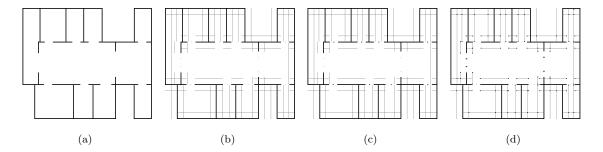
Figure 4: Generation of the roadmap based on ACS-PRM. (a) The original gridmap, (b) adaptive cross C-space sampling, (c) the potential targets (doorways) extracted, and (d) the milestones extracted.
