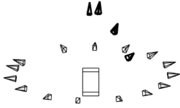
Fig 12 The TempleSparseRing dataset contains 16 “ground-ground” views. The reconstruction is computed inside the box, and is used to predict 4 “air-ground” views (cameras in bold).
