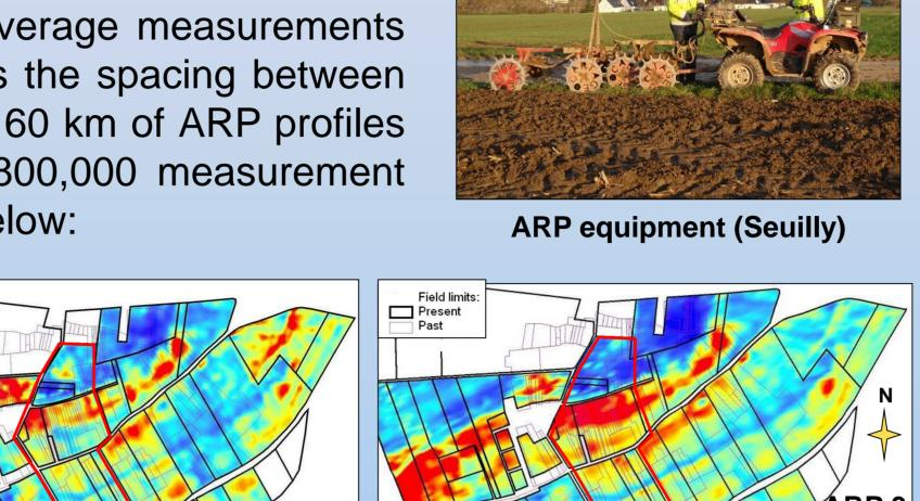
Fig. 3.1: Soil resistivity maps at 3 different depths of investigation
