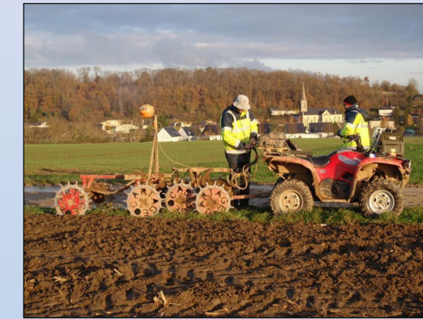
ARP equipment (Seuilly)
