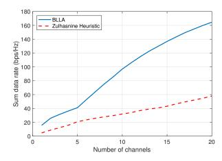
Fig. 8. Normalized sum data rate ( $\alpha=0$ ) as a function of the number of channels using BLLA and the heuristic proposed in [13]. The number of UECs are 5 and UEDs are 95. For BLLA, bounded noise is assumed with  $\ell=5\%$ . For [13], full and exact channel information is assumed.
