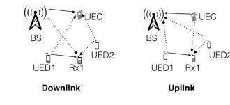
Fig. 1. D2D cellular network layout model.
