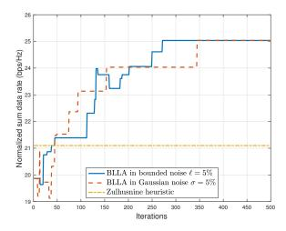
Fig. 5. Normalized sum data rate as a function of the number of BLLA iterations and comparison with the heuristic proposed in [13], for which full and exact channel information is assumed.
