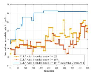
Fig. 3. Normalized sum data rate as a function of the number of BLLA iterations when  ${\cal N}=1.$
