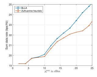
Fig. 9. Normalized sum data rate as a function of the UED power constraint with BLLA and Zulhasnine heuristic [13]. For BLLA, bounded noise with  $\ell=5\%$  is assumed. For the heuristic, full and exact channel information is assumed.
