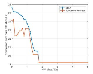
Fig. 10. Normalized sum data rate as a function of the UED rate constraint with BLLA and and Zulhasnine heuristic [13]. For BLLA, bounded noise with  $\ell=5\%$  is assumed. For the heuristic, full and exact channel information is assumed.
