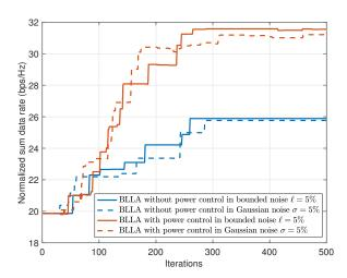
Fig. 6. Normalized sum data rate as a function of the number of BLLA iterations with and without power control.
