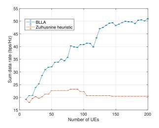
Fig. 7. Normalized sum data rate as a function of the number of D2D users (UED) with BLLA and the heuristic proposed in [13].
