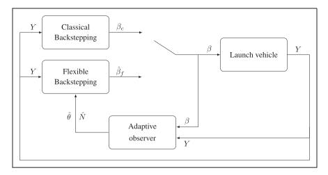
Figure 5. Block diagram of the closed-loop system.
