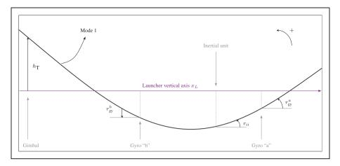
Figure 2. Schematic view of the first mode shape.
