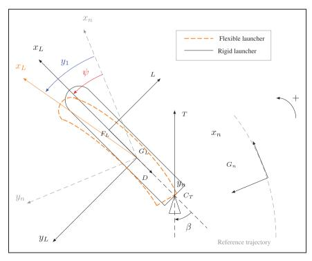
Figure 1. Flexible launch vehicle schematic representation.
