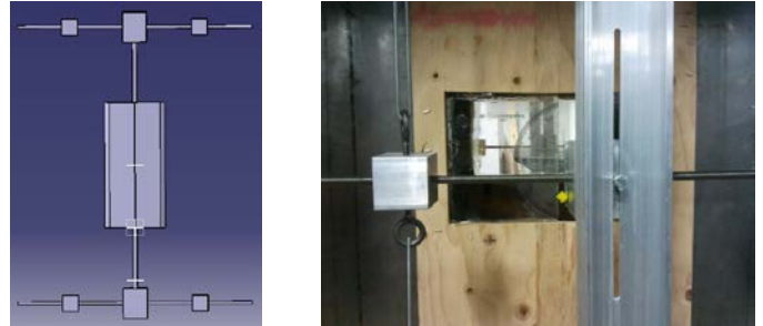
Figure 6 Top view of the deck section with mechanical link (CAD) and restraining system with C-section bar
