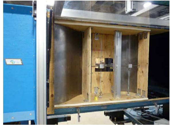
Figure 3 Clarkson University wind tunnel, apparatus mounted inside the test section
