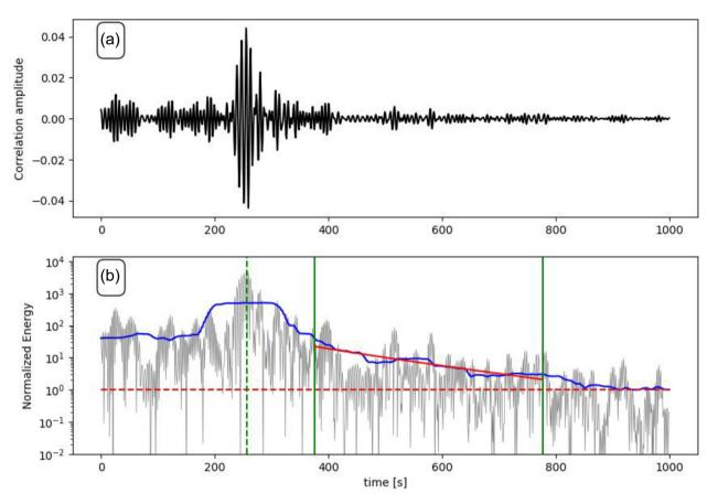
**Figure 3.** Example of processed trace (station couple CH.BERGE—Z3.A263A, interstation distance 703 km). (a) Correlation filtered between 5 and 10 s. (b) Same trace squared (grey) and smoothed (blue). The red line corresponds to the modeled coda decay after inversion for coda-Q. The green lines mark the borders of the interval in which the coda is fitted. Green dashed line: main arrival. Red dashed line: noise level (normalized to 1). Note the logarithmic vertical scale in the bottom plot.
