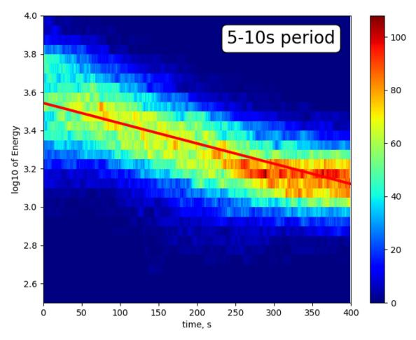
Figure 5. Smoothed energy (log scale) as a function of time (lag time after main arrival), after correction for the  $t^{-\alpha}$  term, for the same traces as in Fig. 4, and for the 5–10 s period band. The traces are shown in the form of trace density where the colour of each pixel indicates the number of traces crossing it. The red line corresponds to the (geometrical) average of coda-Q observed on the same traces.
