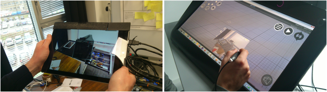
Figure 12. Illustration of the asymmetrical (HWD and WIM) prototype. The agent on the left is guided by the remote expert on the right.
