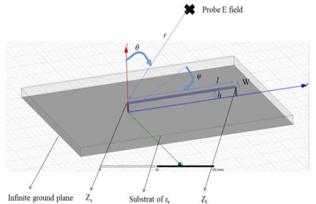
Fig. 4. PCB schematic.
