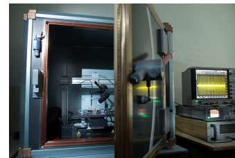
Fig. 1: Test bench for fault attacks by electromagnetic injection.
