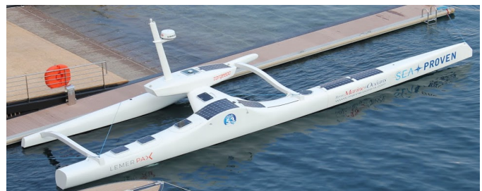
Figure 1. The ASV Sphyrna, 17m long. It is a proa (South Pacific design), consisting of two unequal length parallel hulls. It is extremely stable, even at high wind force.
