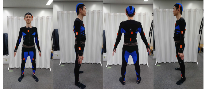
Fig. 3: Sensor positioning. The suit is composed of 34 motion capture markers and 12 IMUs.
