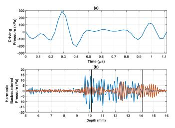
Fig. 4. (a) Optimal transmitted stochastic wave  $\mathbf{x}$  obtained by the genetic algorithm at the transducer output when the prefiltered stochastic waveform  $\mathbf{w}$  is optimal. (b) Harmonic backscattered pressure obtained by pulse inversion and optimal prefiltered waveform. As an illustration, the harmonic RF line in red is obtained by using the better fixed-frequency Gaussian pulse.
