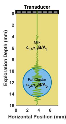
Fig. 1. Grid of properties of the medium constituted of milk (medium 1) with a fat cluster (medium 2): c is the speed of sound wave velocity,  $\rho$  the density and B/A the nonlinearity parameter. The ultrasound transducer was at a depth of 0 mm, here at the top. As an illustration, a harmonic RFline z is depicted in green.
