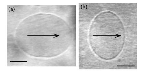
Fig. 1: The two competing shapes of magnetoliposomes subjected to a magnetic field (amplitude  $H_0$ =400 Oe, field direction along the arrow); (a) prolate ellipsoid for a high ionic strength ferrofluid ( $C_s^0$ =85 mM); (b) oblate when the ionic strength has been lowered by dialysis ( $C_s^0$ =7.75 mM). Length of the bar is 10  $\mu$ m.
