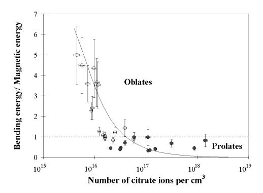
Fig. 3: Ratio of the two competing terms  $E_b/E_m$  in the expansion of the free energy as a function of ellipticity. They are calculated for oblate (open markers) and for prolate (filled markers) liposomes using both experimental data  $(C_p, C_s, R_0)$  and assumed parameters (see text). Solid line is plotted from Eqs. (1) and (10) for typical values  $R_0$ =15 µm and  $\lambda$ =5×10<sup>-3</sup>.
