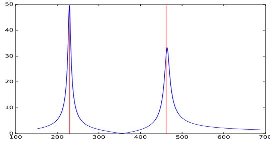
Figure 1: Modulus of the dimensionless input impedance of the resonator with respect to frequency. The two resonances are quasi-harmonic: first resonance frequency  $229\text{Hz}$  (left red vertical line), second resonance frequency  $463.5\text{Hz}$  slightly higher than the octave  $458\text{Hz}$  (right red vertical line), corresponding to an inharmonicity of 0.012.
