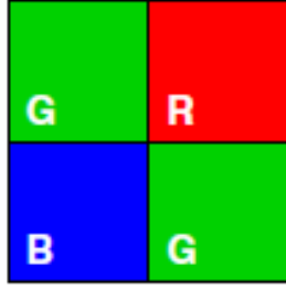
Figure 1: Bayer pattern that can be used in color cameras
