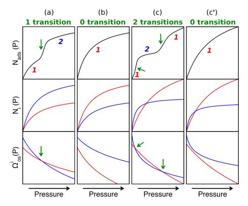
Figure 2: The four possible cases of Langmuir-type adsorption in materials with two metastable phases 1 and 2. Top panels show the adsorption isotherms, middle panels depict the step-free isotherms corresponding to each phase, and bottom panels plot the osmotic potential of both phases. Green arrows indicate guest-induced structural transitions.
