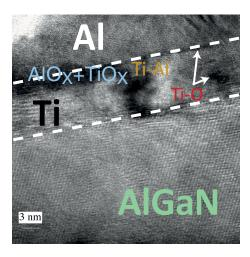
Figure 3. HRTEM image of ohmic contact at the Al/Ti/Al<sub>0.28</sub>Ga<sub>0.72</sub>N interface after rapid thermal annealing forming alloy compositions at 900°C.
