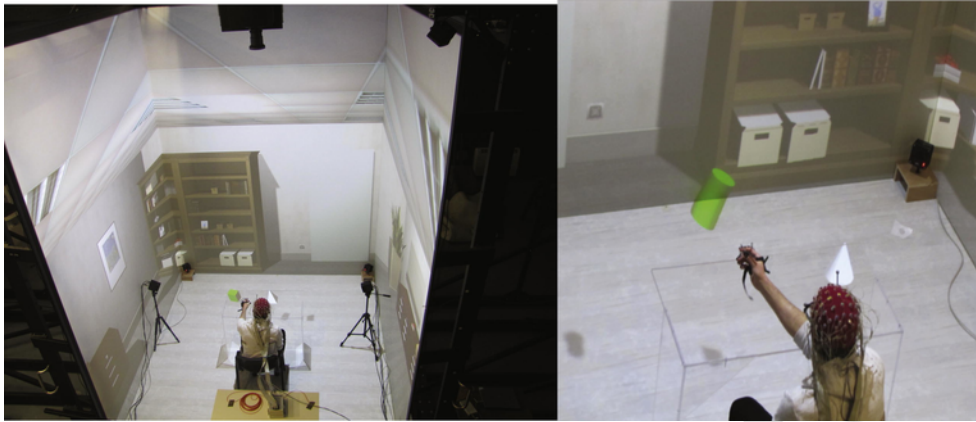
Fig. 1. Participant in the CAVE, wearing a finger-tracker and 3D glasses while manipulating virtual objects.
