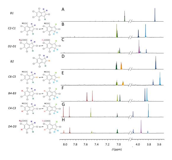
**Figure 3.** Relevant <sup>1</sup>H NMR spectra regions of selected indene-based TP (600 MHz). Data were recorded in  $(CD_3)_2CO$  excepted for B1, recorded in CDCl<sub>3</sub>. The spectral regions  $\delta$ 3.5-4.1 ppm and  $\delta$ 6.8-8.1 ppm are shown for B1 (A), C1-C2 (B), D1-D2 (C), B2 (D), C5-C6 (E), B3-B4 (F), C3-C4 (G), D3-D4 (H).
