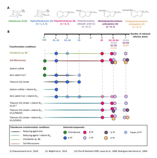
**Figure 2**. Chlordecone TP (A) Five families of observed chlordecone TP (B) Chemical conditions for chlordecone degradation and released of one to seven chloride atoms. 8-monohydrochlordecone was assigned to A2. A3 and A4 correspond to dihydrochlordecones, and A5 to a trihydrochlordecone.
