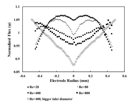
Figure 5: The evolution of the normalized flux,  $\varphi$ , (the ratio between the mass flux, j, and the average flux  $j^*$ ) at the electrode surface with the variation of the velocity inside the cell represented by the Reynolds number Re.
