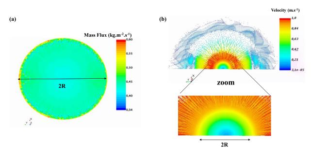
Figure **-b**, on a plane parallel to the electrode surface. An inset magnifies the vectors field to illustrate the symmetric and uniformity of the flow in the boundary layer.
