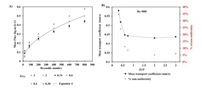
Figure 6: Variation of Mass flux with the Reynolds number for different nozzle-electrode distance 'Z', which ranges from 0.2 mm to 1.5mm, presented as the ratio of Z by the nozzle radius  $r_{,}$  (Z/r), and B) represents the plot of the variation of the mass transport coefficient and the % of the uniformity with the variation of the ratio of Z/r at Reynolds number 800.
