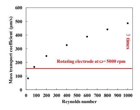
Figure 10: Comparison of the transport in the two different geometries: horizontal line corresponds to RDE at maximum reliable rotation rate 5000 rpm corresponds to Re=3500, the closed circle symbol corresponds to the numerical results of the new designed jet cell.
