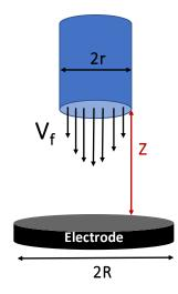
Figure 1: A schematic presentation of the geometrical parameters of a jet electrode: r is the nozzle radius, R is the electrode radius, Z is the nozzle-electrode distance,  $V_f$  is the volume flow rate. The electroactive surface is represented in a darker shade of gray.
