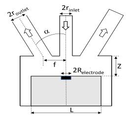
Figure 2: Geometric scheme of the inlet (r) centered above the electrode of radius R with two symmetric outlets ( $r_o$ ) aligned at angle  $\alpha$ =26° with the inlet, the chamber, Z, represents the distance between the inlet and electrode surface
