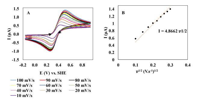
Figure 8: (A) Cyclic voltammograms of the (1mM)  $Fe(CN_6)^{3-}/Fe(CN_6)^4$  in an electrolyte of 0.5 M NaCl at a range of scan rates (10mV/s to 100 mV/s), and (B) Peak current as a function of scan rate, with the linear relationship (dotted line). The experiments were conducted at room temperature.
