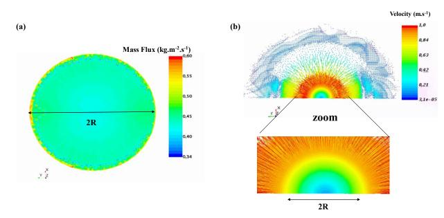
Figure : a) Mass flux at electrode surface, and b) Velocity vectors at a plane parallel the electrode at distance of mm with zoom on electrode area. This numerical result corresponds for the  $r_T/R=1$ ,  $Z/r_T=0.74$ , Re=800.
