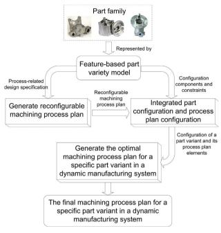
Fig. 1. A solution framework for RMPP.
