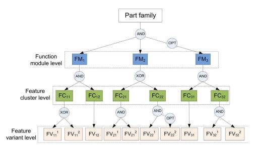
Fig. 5. Illustration of a variety decomposition network.
