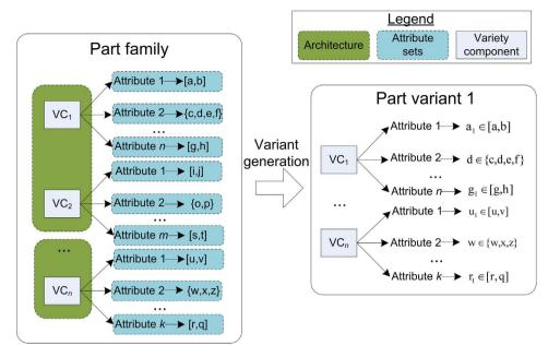
Fig. 2. Illustration of the concept of part family.
