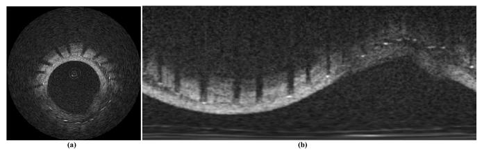
Fig. 3. (a) typical slice image as delivered by the OCT device, (b) polar reformation of the image in (a); the horizontal and vertical axes represent respectively the angular position between 0 and 360 degrees and the pixel position from image center (probe position) to image border.
