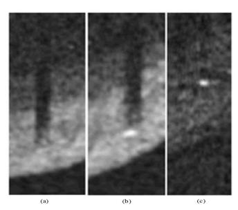
Fig. 5. Typical strut appearances in OCT acquisition: (a) a shadow zone is visible but no strut echo; (b) both shadow zone and strut echo are visible; and (c) a strut echo is visible but no shadow zone.
