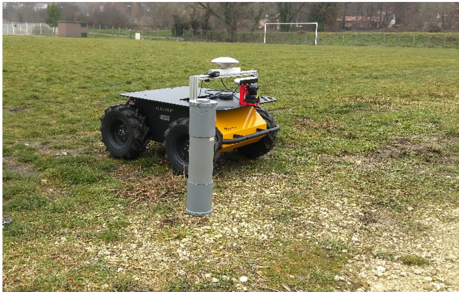
Figure 10. All-terrain mobile platform running ASAWoO next to the base station kit
