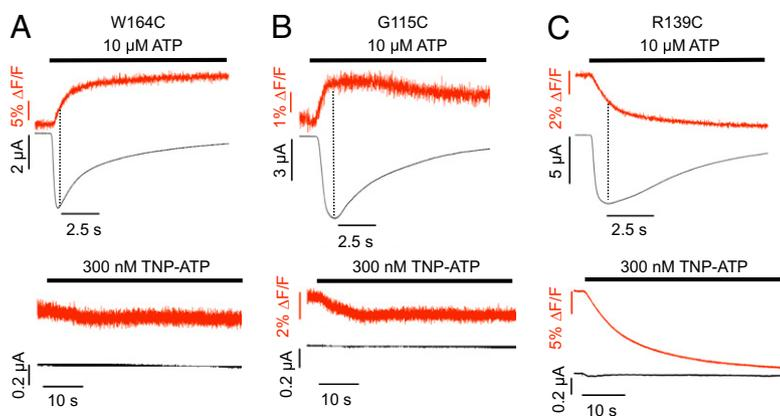
**Fig. 4.** Current traces and fluorescence changes of TMRM-labeled mutants that were rationally planned based on a homology model. Recordings were made on application of agonist (10  $\mu\text{M}$  ATP) or antagonist (300 nM TNP-ATP). (A) W164C, (B) G115C, and (C) R139C. Dotted lines indicate the current peak times.
