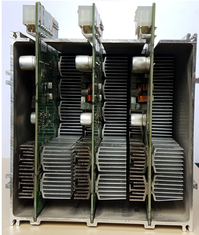
Fig. 7. An AntMiner S7 from Bitmain (side view without the fan). The three hashboards are visible.
