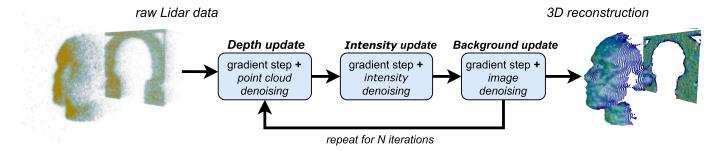
Figure 2: Block diagram of the proposed real-time framework. The algorithm iterates between depth, intensity and background updates, applying a gradient step followed by a denoiser. Each step can be processed very quickly in parallel, resulting in a low total execution time.
