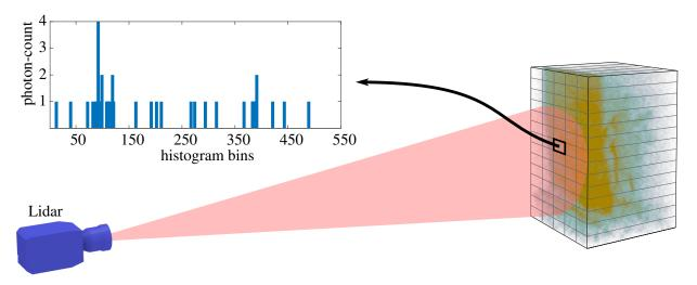
Figure 1: Illustration of a single-photon lidar dataset containing two surfaces (the man behind camouflage from [15]). The graph on the left shows the histogram of a given pixel. The limited number of collected photons and the high background level makes the reconstruction task very challenging. In this case, processing the pixels independently yields poor results, but they can be improved by considering *a priori* knowledge about the scene's structure.
