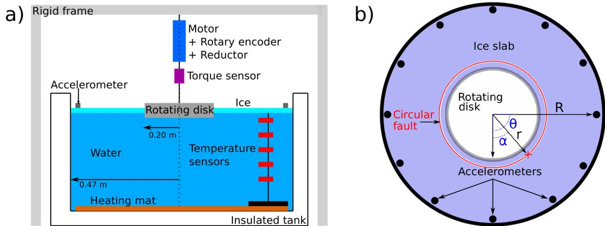
**Figure 1.** Schematic a) Side-view and b) top-view, of the experimental setup. The fault and accelerometer circle radii are denoted  $r$  and  $R$ , respectively.  $\alpha$  and  $\theta$  denote a rupture and an accelerometer angular positions, respectively.
