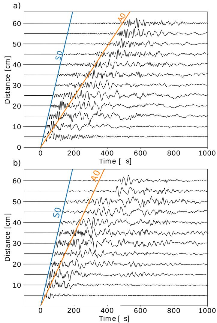
**Figure 2.** Normalized waveforms recorded at different distances from the source for a floating ice plate of thickness a) 3 mm and b) 9 mm. The source is of Nielsen-Hsu type, which is commonly used in acoustic-emission testing. Lines refer to the theoretical S0 (blue) and A0 (orange) propagation modes in vacuum. The origin time  $t = 0$  s is the time of the source.
