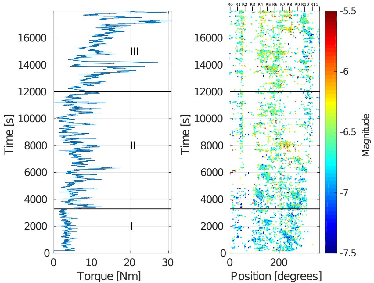
**Figure 5.** Left: Torque measured for the imposed velocity of  $1.6 \times 10^{-4} \text{ m.s}^{-1}$  at  $-10^\circ\text{C}$ . The initial rupture that creates the fault is not shown,  $t_0$  represents the time immediately after this rupture. Right: Space and time distribution of the detected ruptures. The color scale represents the magnitude. R0, R1, ..., R11 labels represent the accelerometers positions.
