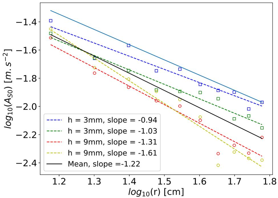
**Figure 3.** Maximum amplitude of the QS0 mode,  $A_{50}$ , as observed experimentally as a function of the distance to the source,  $r$ , for a 3 mm (squares) and 9 mm (circles) thick ice. Dashed-lines are the best linear fits for each data-set and the solid line is the best fit of all data-points.
