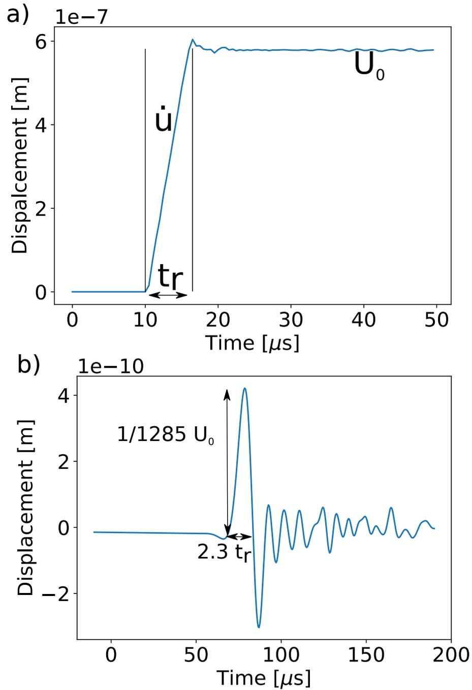
**Figure 4.** Far-field displacement due to a shear dislocation modelled using the COMSOL software. a) Horizontal displacement  $U_0$  imposed on the rupture defined as a  $1 \text{ cm} \times 1 \text{ cm}$  dislocation, with rupture velocity  $V_r = 1675 \text{ m.s}^{-1}$ , sliding velocity  $\dot{u} = 0.1 \text{ m.s}^{-1}$  and rupture duration  $t_r$ . b) Vertical displacement modelled at a distance  $r = 0.25 \text{ m}$  from the source.
