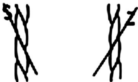
Fig. 4 Schematic representation of yarns spun with a clockwise (Z-spun) and anticlockwise (S-spun) twisting
