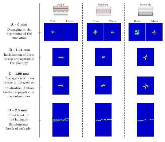
Figure 13: Scenario of damage propagation during a quasi-static tensile simulation on a  $2.25~{\rm J}$  impacted sample of G0C45C0
