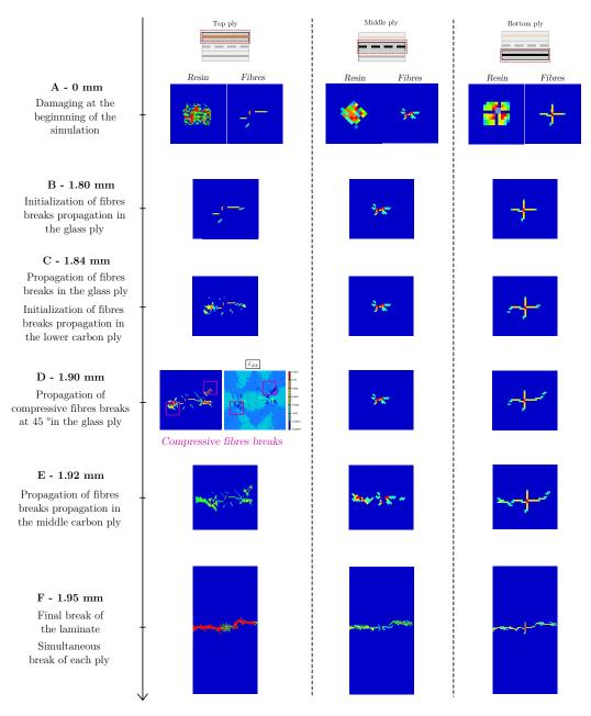
Figure 11: Scenario of damage propagation during a quasi-static tensile simulation on a  $4~{\rm J}$  impacted sample of G0C45C0
