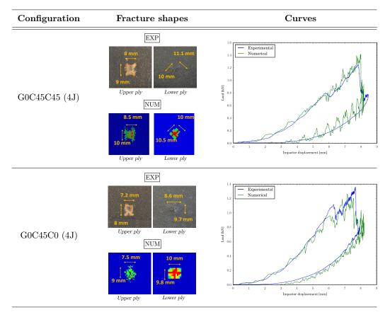
Figure 8: Drop weight impact results on hybrid laminates - Experimental and numerical comparaison
