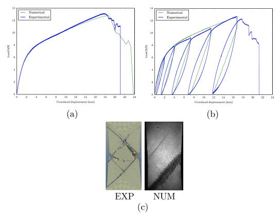
Figure 4: Comparison of numerical and experimental results after (a) normal (b) cycled quasi-static tensile tests on two plies of carbon woven at  $\pm 45^{\circ}$
