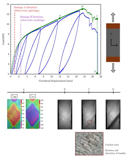
Figure 2: Emergence and progress of shear damage during a quasi-static tensile test on two plies of carbon/epoxy woven  $\pm 45^\circ$
