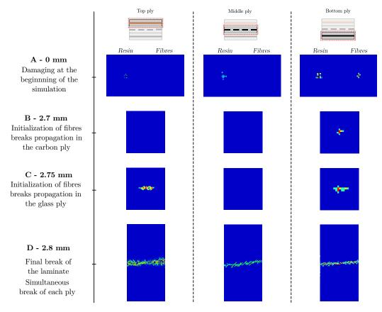
Figure 12: Scenario of damage propagation during a quasi-static tensile simulation on a  $1~{\rm J}$  impacted sample of G0C45C0
