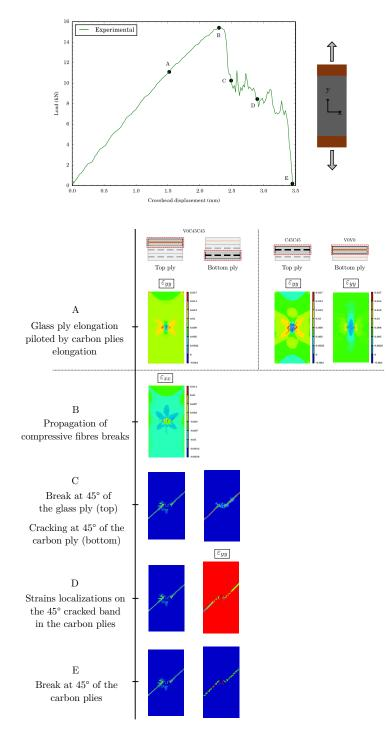
Figure 10: Scenario of damage propagation during a quasi-static tensile simulation on a  $4~{\rm J}$  impacted sample of G0C45C45
