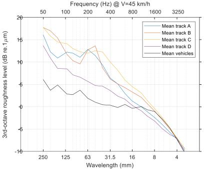
Figure 7: Comparison of wheel and rail roughness spectra as a function of wavelength and frequency
