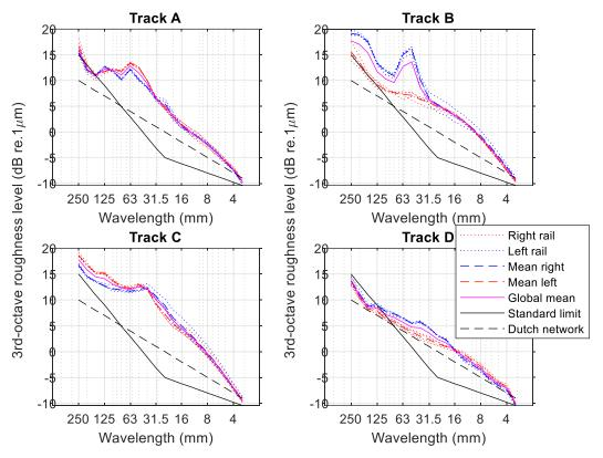
Figure 4: Rail roughness spectra measured on test tracks
