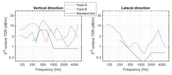
Figure 9: Track Decay Rates (TDR) measured on test tracks D and B
