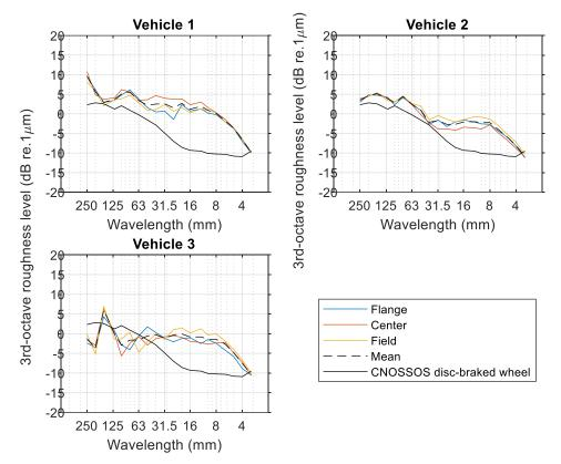
Figure 6 : Wheel roughness spectra measured on test vehicles
