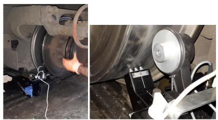
Figure 5: Wheel roughness measurement system
