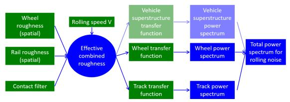
Figure 1: CNOSSOS rolling noise model for rail-bound vehicles (inputs in green, outputs in blue)
