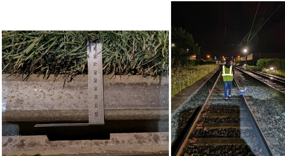
Figure 3: Identification of the width of the running band on the railhead and measurement with the CAT
