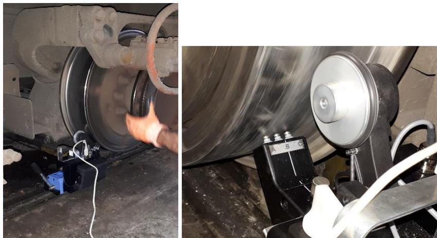
Figure 5: Wheel roughness measurement system
