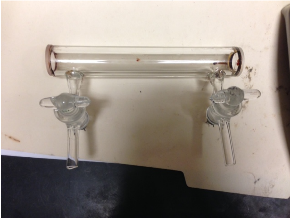
Figure S.21: A photograph of the gas IR cell.
