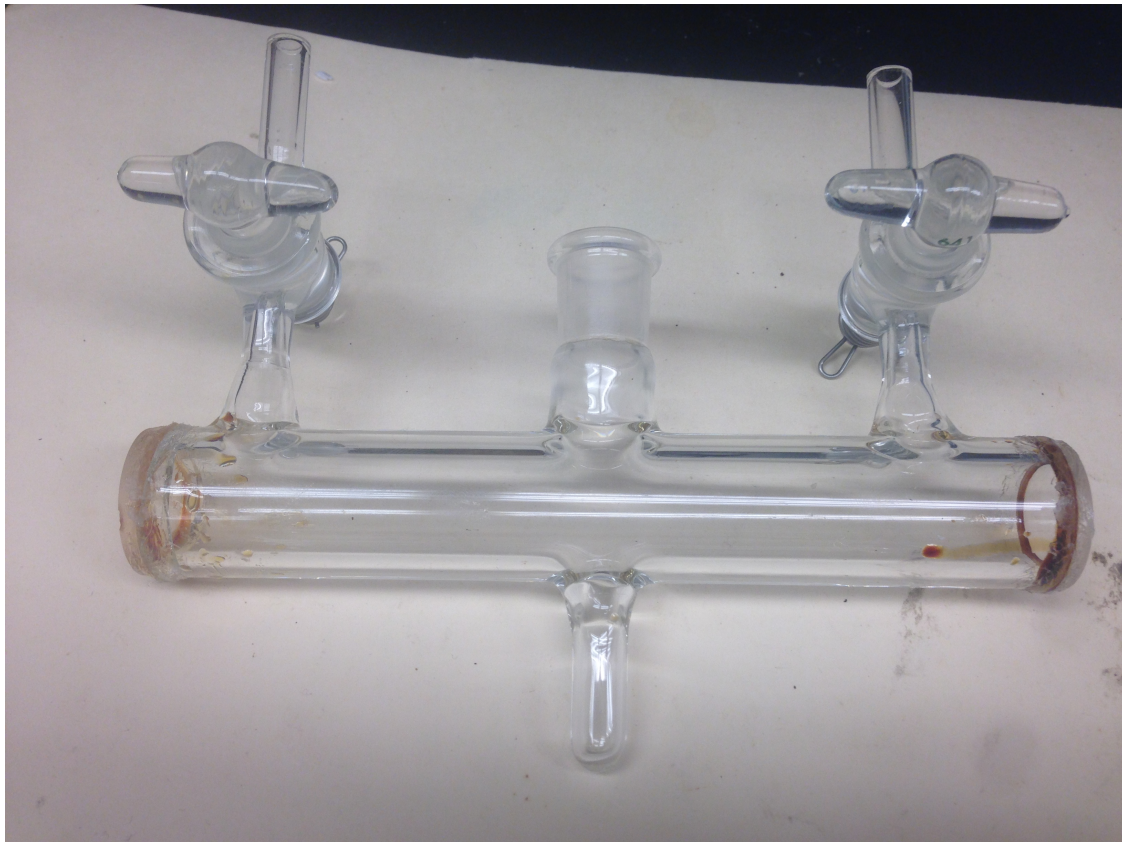
Figure S.22: A photograph of the modified gas IR cell used for the generation and analysis of gases evolving from a solid sample (placed into the glass pocket) by thermal decomposition.
