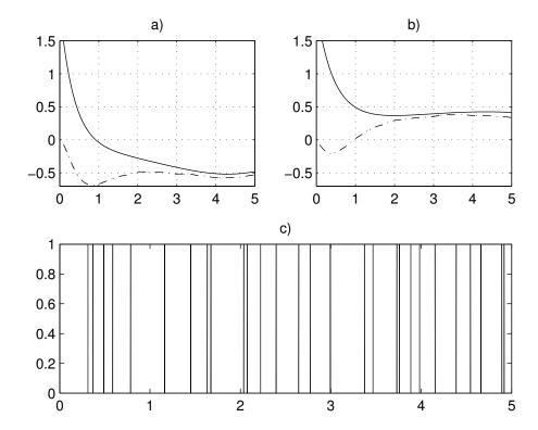
Fig. 1. a) unmeasured state  $x_2$  (solid line) and estimation  $\hat{x}_2$  (dashed line) b) unmeasured state  $x_3$  (solid line) and estimation  $\hat{x}_3$  (dashed line). c) Sampling instants indicated by vertical lines.
