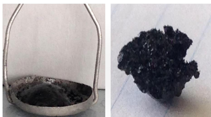
Figure 4: images of the char formed during TGA analysis (under air) of Phyt/PEI-TA.
