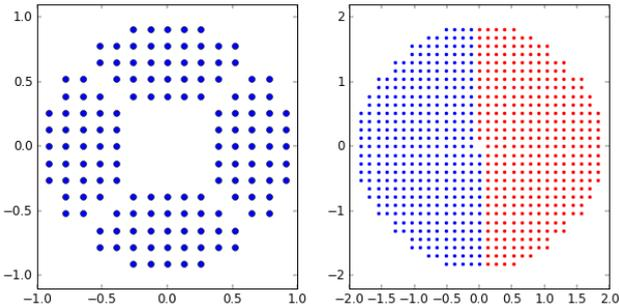
**Fig. 2.** Discrete representation of the HST for kernel analysis of the NICMOS images. *Left panel:* representation of the pupil model defined by the cold mask of the instrument. The model takes into account central obstruction and spider vanes, but neglects finer structures such as support pads. The grid pitch is 0.13 m, the outer diameter is 1.95 m, the inner diameter is 0.71 m, and the thickness of the spider vanes is 0.07 m. *Right panel:* corresponding uv-plane coverage.
