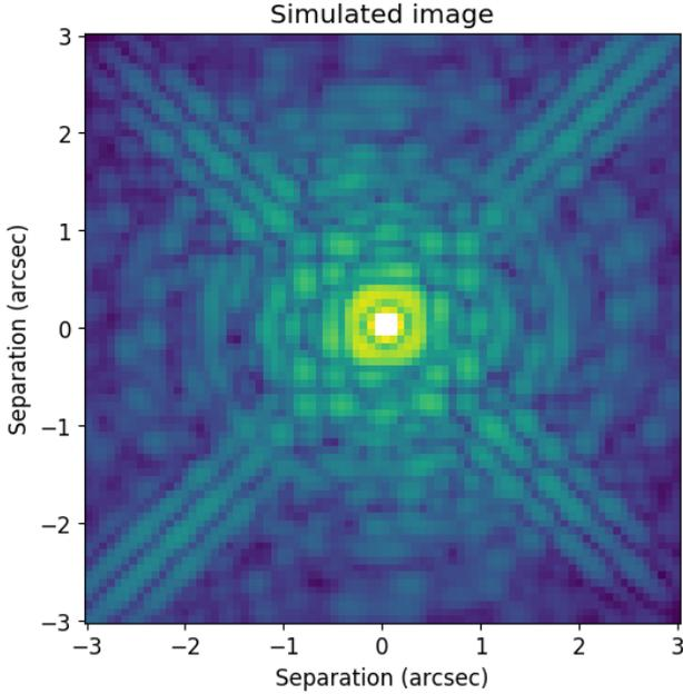
**Fig. 1.** Example of a simulated HST NICMOS2 128 s image through the F222M filter ( $2.22 \mu\text{m}$ ) including shot, readout noise, and saturation. The plate scale is 76.5 mas per pixel and the image also features a companion at  $10^3$  contrast located 450 mas to the left and 450 mas below the primary. The clipped value of nine pixels at the core of the PSF (displayed in white) would usually prevent the use of Fourier analysis.
