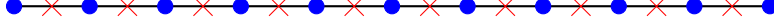
FIGURE 1. The red crosses stand for the centered grid while the blue dots are for the staggered grid
