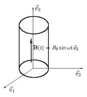
**Figure 4.** Free cylindrical sample and sinusoidal magnetic induction loading.
