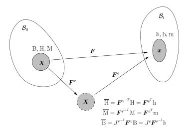
**Figure 1.** Illustration of the multiplicative decomposition  $F = F^e F^v$  and transport of the magnetic field vectors on the intermediate configuration.
