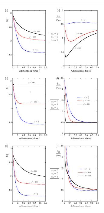
**Figure 3.** (a) (c) (e) Dimensionless magnetic field evolution  $\overline{H}(\tilde{t})$  and corresponding (b) (d) (f) dimensionless total stress  $\widetilde{\sigma}_{33}(\tilde{t})/\mu_{\rm neq}$ . In each case, only one non equilibrium magnetization parameter is activated:  $\alpha_4$  for (a-b),  $\alpha_5$  for (c-d), and  $\alpha_6$  for (e-f). Three different ratios  $\beta=2/3,4.67$ , and 500 are used for each calculation. Prepared using sagej.cls
