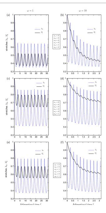
**Figure 5.** Total and viscoelastic stretches  $\lambda_3(\tilde{t})$  and  $\lambda_3^{\rm v}(\tilde{t})$  in response to applied sinusoidal magnetic induction with frequency  $\omega=1$  in (a) (c) (e), and  $\omega=10$  in (b) (d) (f). Each time with the activation of different magnetization parameters, as indicated.
