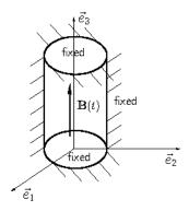
Figure 2. Fixed cylindrical sample and magnetic induction loading.
