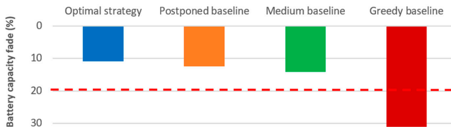
Figure 10. Battery capacity loss during 10 years of operation.
